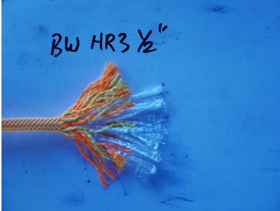
1/2" Bluewater HR3; Blend of Polyester and Polypropylene sheath; polypropylene core
